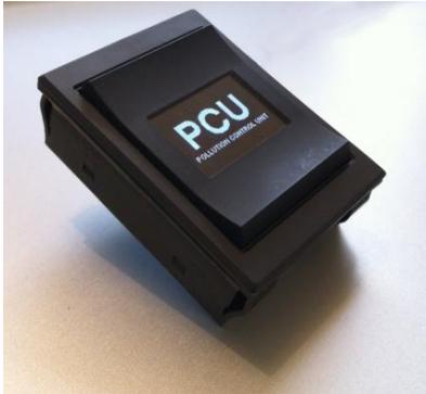
The HMI for the PCU filter pressure monitor is a “Smart” rocker switch with a built in organic LED monochrome graphic display. The rocker switch has 3 momentary switches, one is actuated when the top portion of the rocker is depressed, the second one is actuated when the middle portion of the rocker is depressed, and the third is actuated when the bottom portion of the rocker is depressed. This configuration allows for navigation through menus and making selections.
